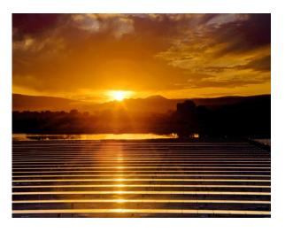
**Glare:** A continuous source of brightness, relative to diffused lighting. This is not a direct reflection of the sun, but rather a reflection of the bright sky around the sun. Glare is significantly less intense than glint.
