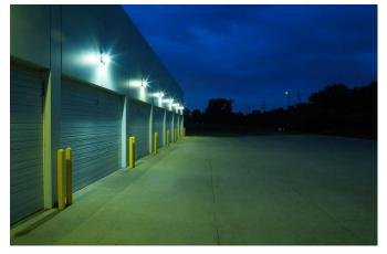
**BEFORE:** Many HID sources like high pressure sodium or mercury vapor provide poor color rendering and non-uniform distribution.
