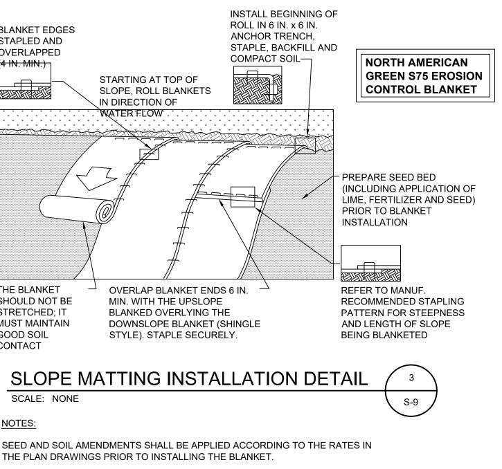
PROVIDE ANCHOR TRENCH AT TOE OF SLOPE IN SIMILAR FASHION AS AT TOP OF
